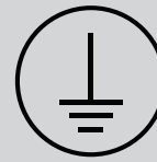
earthing wire (provided by installer)
