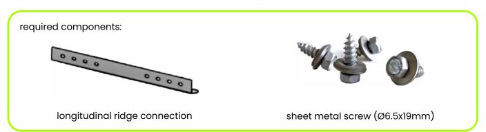
In the longitudinal ridge connection, one L-profile is placed on each rail. These are attached on top of both rails with two sheet metal screws (Ø6.5x19mm) per rail.
