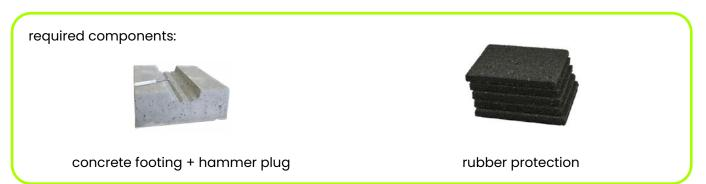
Concrete footings are placed under the full length of the connected basic units. A footing is placed at the beginning and the end of the connected basic units. A rubber is always placed under the concrete footings to protect the roof surface. At least 5mm of rubber must be visible on each side of the concrete footing.
