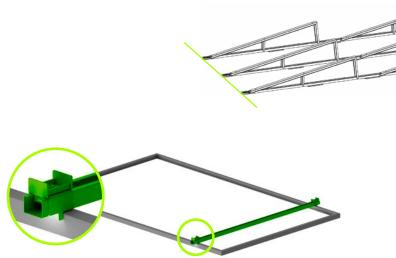
Set the width of the panel on the spacer.
