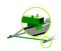
Turn the spacer 180° and align the rows.
