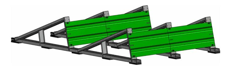
Place the backplate on the back of the assembly triangle and attach it with at least 4 sheet metal screws (Ø6.5x19mm).
