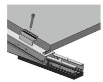
Fix the clamps into the screw thread provided in the assembly triangles with the M8 bolts. Screw the bolts hand tight. After the complete solar module array has been assembled, tighten the bolts with minimum 19Nm and maximum 25Nm. (see general notes)
