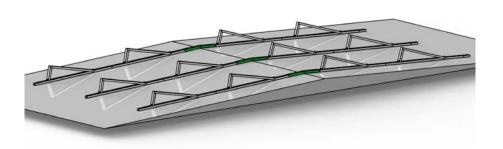
In the transverse ridge connection, the ridge profile is placed over the ends of the rails. The ridge profile can be folded in the middle to the appropriate slope. It is then attached to the basic units with 8 self-drilling screws (Ø5.5x25mm).
